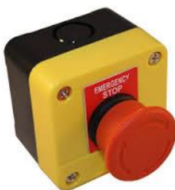
FIG.8. Emergency Stop Button. The button must be coloured red and if a background is present it must be coloured yellow.
