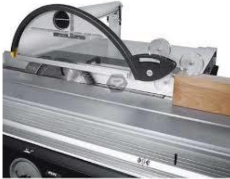
FIG.3. The hood guard on this Panel saw is an example of adjustable guarding. This guarding requires adjustment by the operator
