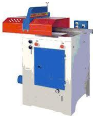
FIG.2. The tunnel guard (Removable) and bottom housing (Permanent) on this Docking saw are examples of close proximity fixed guarding
