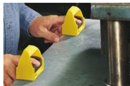
FIG.10. Two handed operation featuring button shrouds
