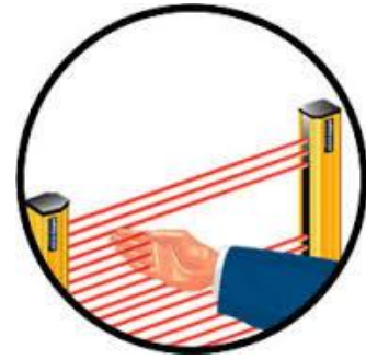
FIG.6. Photoelectric guarding will automatically shut down a machine when the curtain is broken
