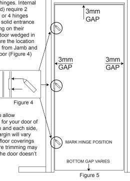
Place door securely on its side and transfer all measurements marked for hinges onto side of door. Using the hinge as a template trace around the hinge (Figure 6).
