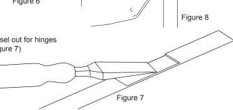
Stand your door in the frame to check hinge locations are correct. Using wedges adjust the door to locate the correct hinge position and screw into place.
