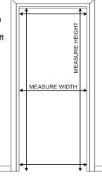
Transfer your door opening measurement measurements taken in step 1 to your new Hume door. Your door may require trimming to fit the opening. A maximum of 3mm may be trimmed from any edge. Figure 2 shows a power planer used to trim door.
